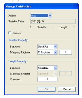
■ Ignore the function code (FF) of the response: (\*, 1): Ignore the word whose length is 1. If the user wants to store the function code, the user can refer to the setting of the device address (IA) to store the function code in the D register.
