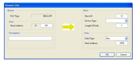
After the setting is complete, the user can designate the communication port used in Modbus Advance — COM port 2 on left-side module number 1.
