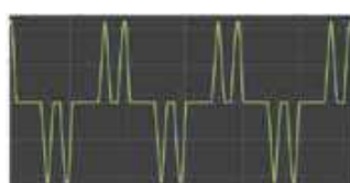
Motor drive without DC choke THDi 107%
